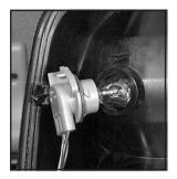
4. Pull the bulb straight out from the socket.
